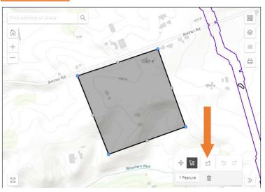
When you click on the Sketch Widget, it opens a new window to draw the survey boundary. Several map tools will be visible in the lower left corner of the screen.
